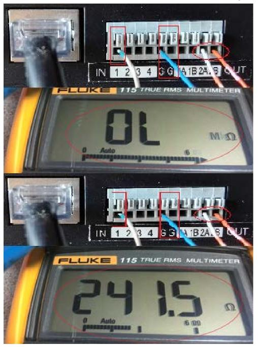
Figure 25-4: GVR355X Alarm\_Out Circuit Measurement
