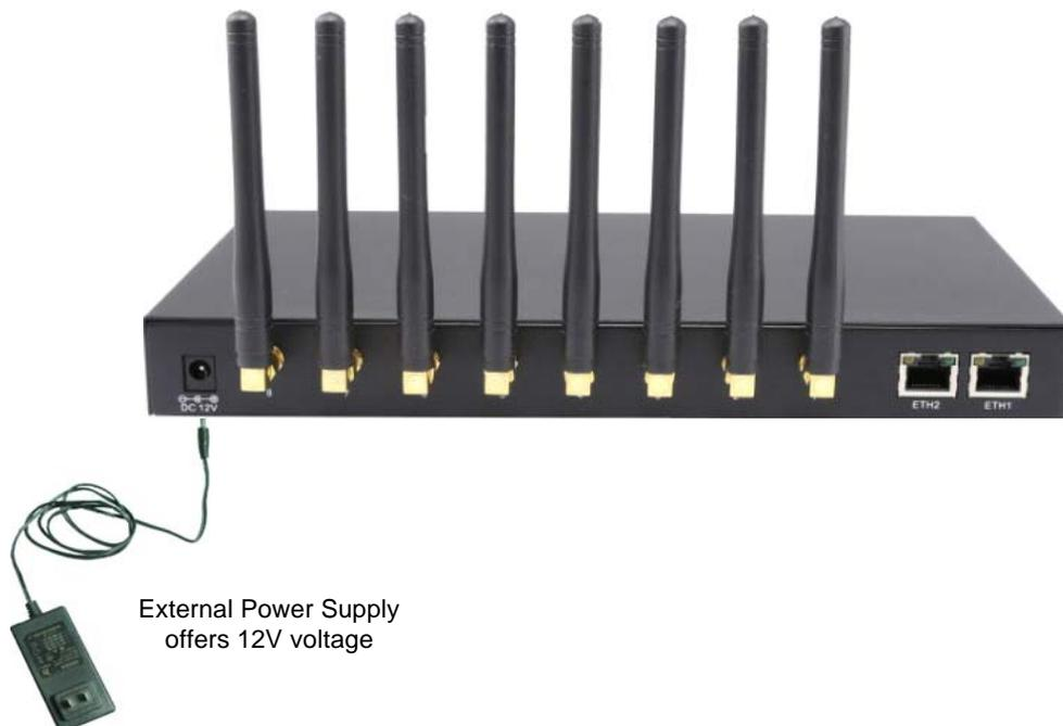
Figure 2-1 Wireless Gateway Power Connection
