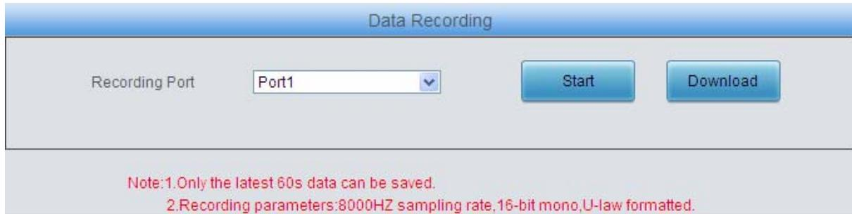
Figure 3-112 Data Recording Interface
