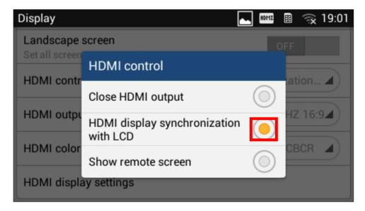
Figure 151: Settings->Display->HDMI Control
